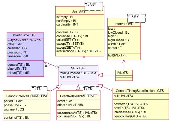
Figure 13: Overview of Timing Specification Data Types
