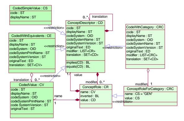
Figure 3: The Concept Descriptor information model. The concept descriptor is mostly used in one of its restricted or "profiled" forms, CS, CE, CV, and CC.
